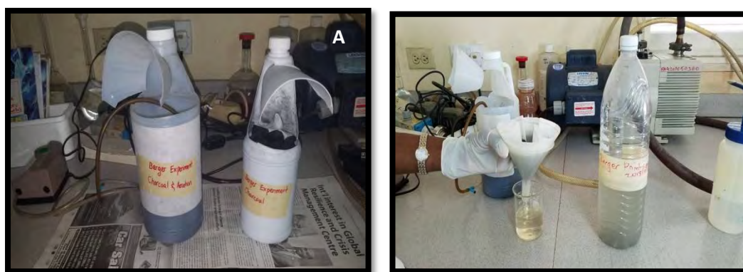
Figures 12A and 12B. Experimental setup up for Berger Paints Limited samples, using charcoal
